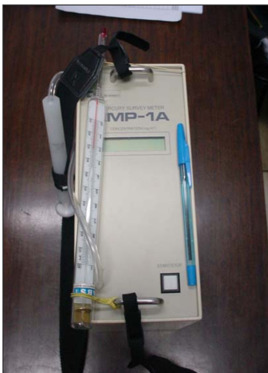
Figura 11. Analisador de Hg no ar, fabricante Nippon Instruments Corporation.
